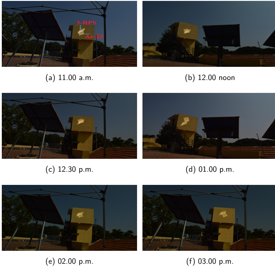
Fig. 21: Deviation of image from the aim-point
